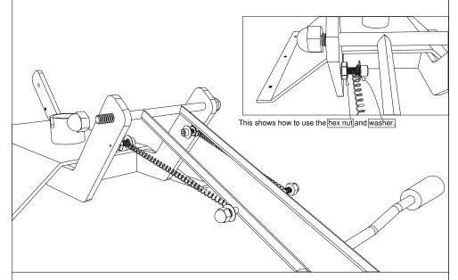
4. Bolt in the bottom bracket using six medium bolts and the six large washers/lockwashers.
