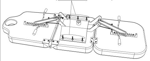
5. Put the adjustment bars in the metal grooves and attach the groove covers using the 4 short flathead bolts and 4 small washers and lockwashers.
