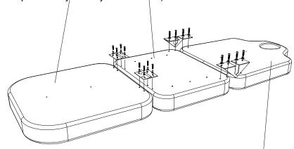
Use 8 medium bolts and 8 medium washers and lock washers with the angled hingesto connect the middle piece to the head piece. (These pieces may already be attached.)
