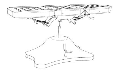
7. Reach in the back and use the single xL bolt and lockwasher and the last large washer to secure the hydraulic.
